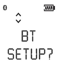
1. Press the ▲ button to enable or disable the Bluetooth communications device (ON/OFF).
